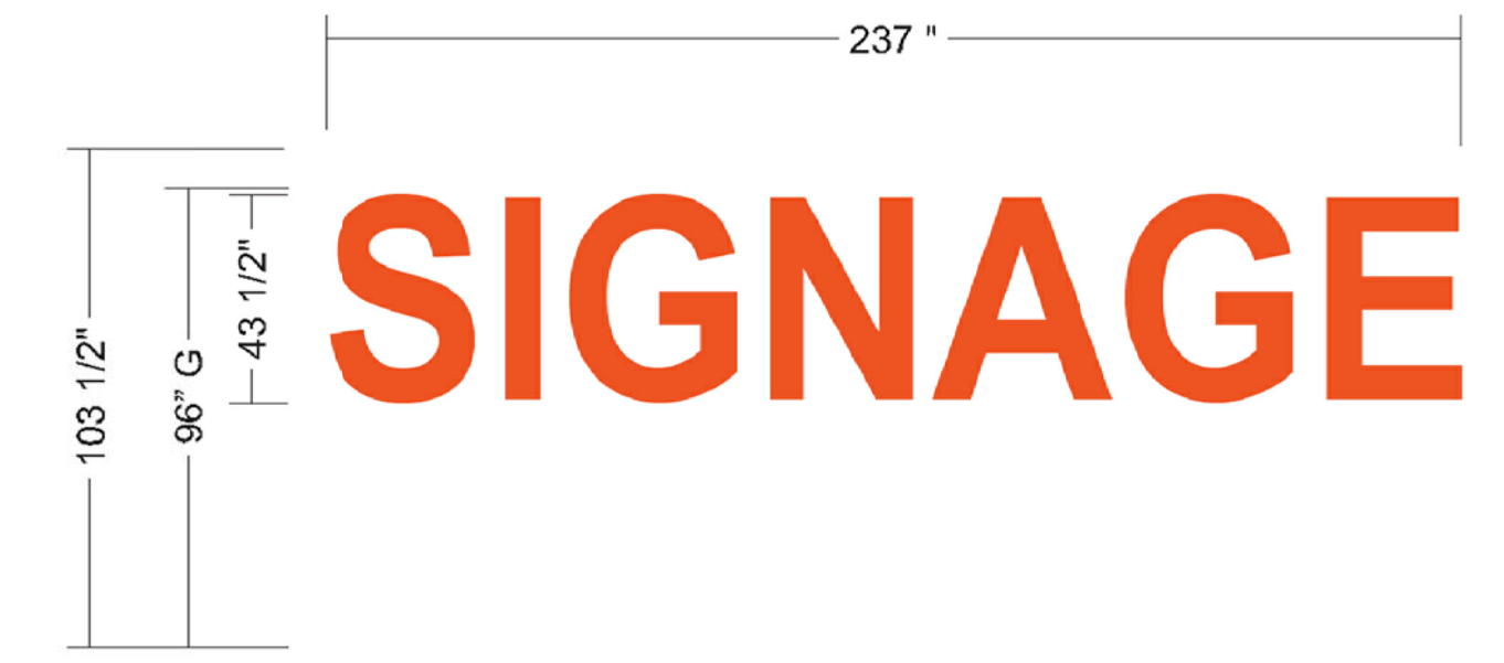
ONE (1) SET OF MINIMUM 3" DEEP INTERNALLY ILLUMINATED LETTERS WATER DROP IS FACE LIGHTED
